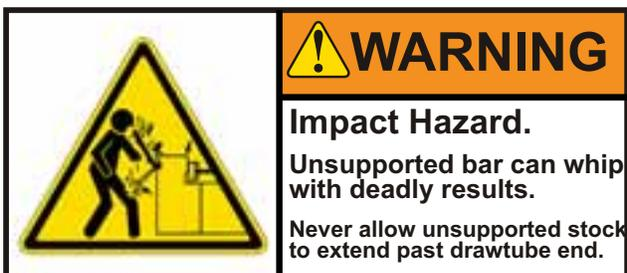
This label is found on front of machine at far left, and on left side removable panel.
