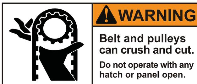
This label is found on front of machine by removable hatch, and on the left side removable panel.
