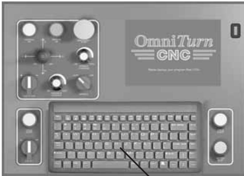
← USB Stick for program storage. **USB must be installed before power-on.** Do not remove USB while powered up.
