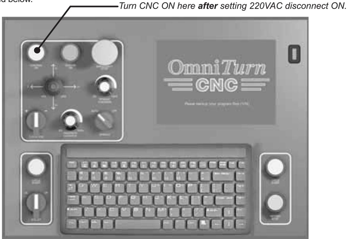
After boot-up, the first screen you see will ask you to back-up your program files. Always select “Y” to backup. Only those programs which have been edited will be copied to the USB stick installed in socket on front-panel of CNC control. Programs will be backed up to USB memory stick (supplied) in the Programs folder. Before a new USB stick is used, you should create a Programs folder on it to maximize program storage.
